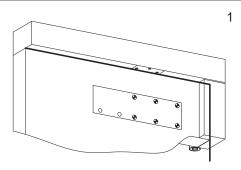
Using the templates provided, mark and drill pilot holes into the door and frame.
