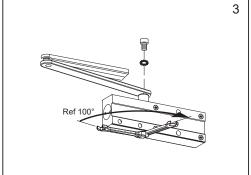
Rotate the bottom pinion to approximately  $100^{\circ}$  with a wrench as illustrated and then assemble the main arm.
