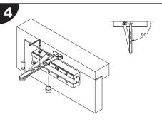
Connect the armset ensuring the pre-loading requirement has been completed.
