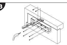
Using the templates provided, fix the mechanism to the door as well as the armset and any necessary brackets.
